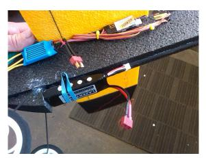
Use a Lipo safe bag or fire proof container when charging ..If the Battery is "puffed up" properly dispose of it Be very careful!
