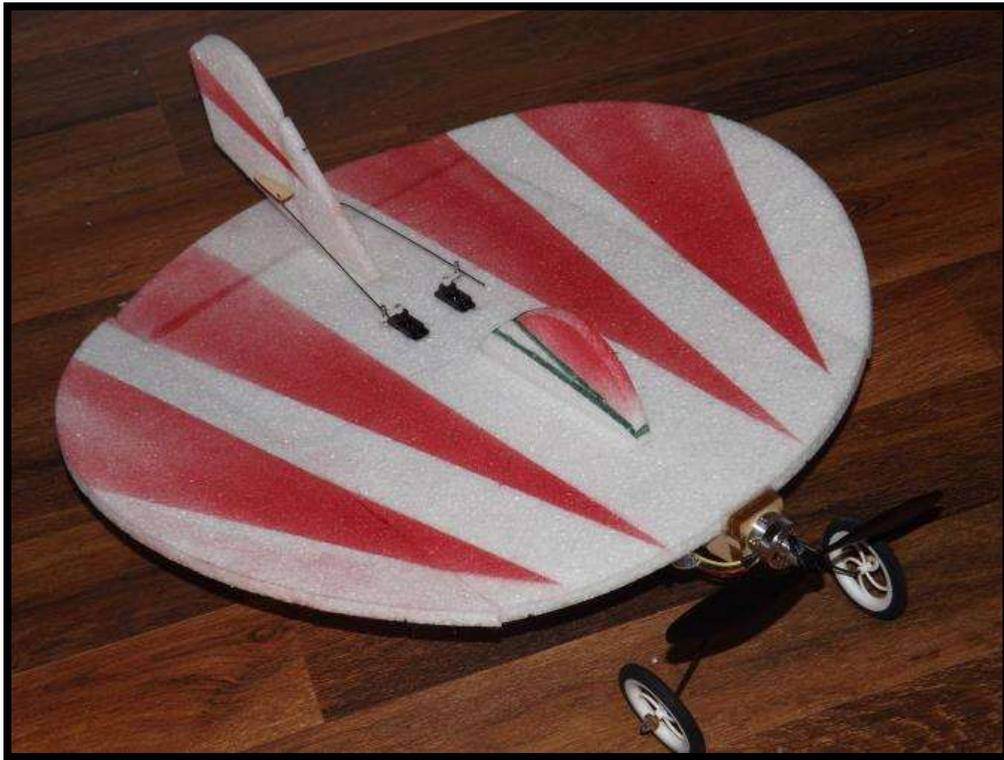
Use velcro to hold the battery in and move the CG. The CG is 5" from the motor mount.
