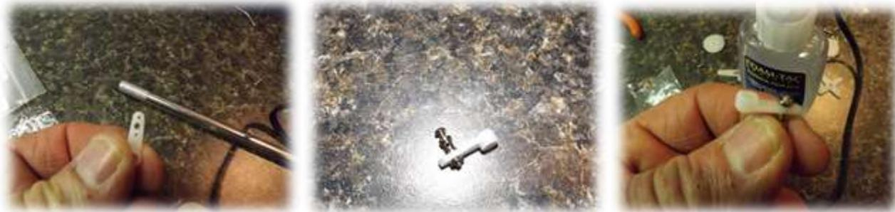
Place the Linkage stopper in the hole and hand tighten the nut and glue in place
