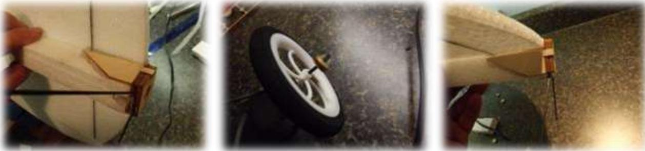
Place the control horns in place after the hinges are completely set and Glue in place
