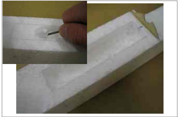
Step 12: Cut around the line drawn on the fuselage, make criss cross cuts in side the pattern. Use a small screwdriver to pick out the foam, bit by bit until the receiver and ESC fit well.
