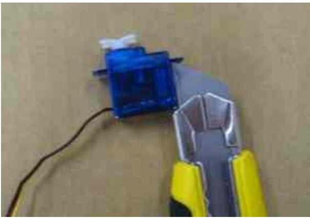
Step 17: Measure the depth of your servos from the bottom to the servo lugs as shown.
