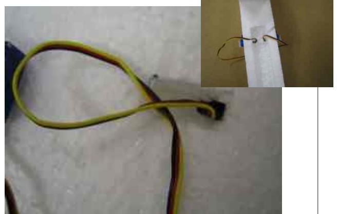
Step 20: Feed the servo plug through to the radio compartment. Seat the servo in the hole and glue the lugs with CA glue.
