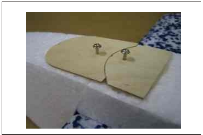
Step 10: Glue on the other plate, lined up with the front plate as shown, attach self tapping screws leaving 3mm proud.
