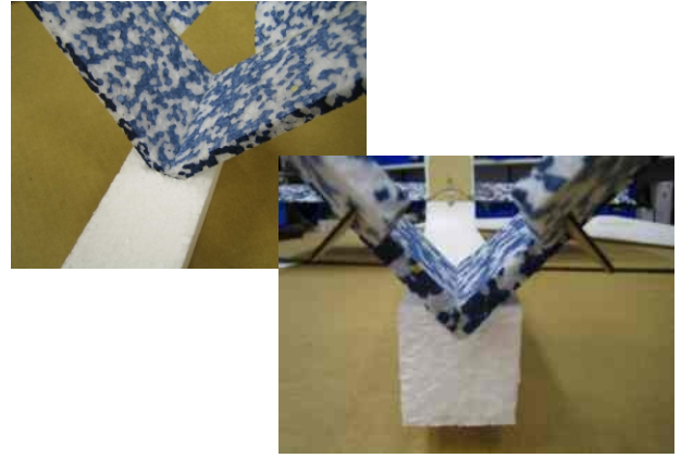
Step 16: Glue in the tail assembly into the V cut in the rear of the fuselage, with the elevators facing rearwards.
